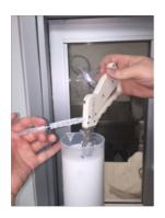
Suggested: Submerge device in container. While submerged, squeeze handle to disperse lubricant throughout the mechanism.
