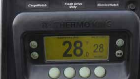
Trailer temperature monitoring equipment
